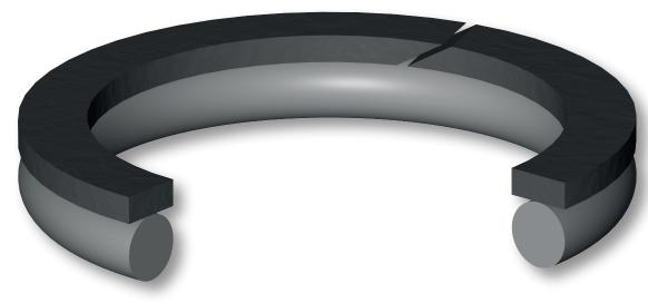
The function of ring type Aston Seals BRT is to avoid the extrusion and damage of the O-Ring that normally occurs in the presence of large gaps or high pressure.
