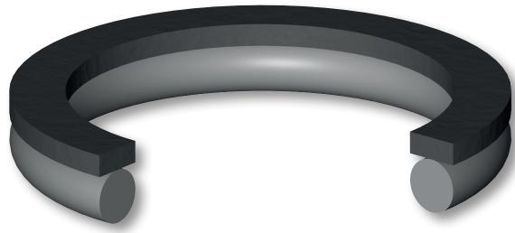
The function of ring type Aston Seals BRC is to avoid the extrusion and damage of the O-Ring that normally occurs in the presence of large gaps or high pressure.
