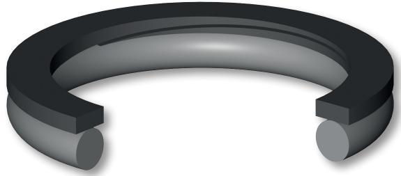
The function of ring type Aston Seals BRA is to avoid the extrusion and damage of the O-Ring that normally occurs in the presence of large gaps or high pressure.
